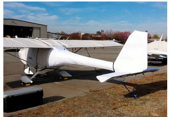
Remos Empennage Cover (test fit cover)
