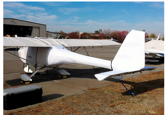
Remos Empennage Cover (test fit cover)
