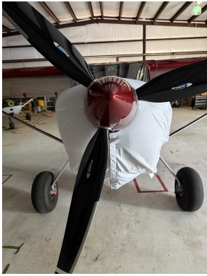
Rans S-21 Engine Cover, test fit cover
