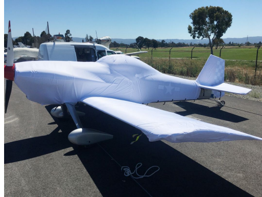
Van's RV-3 Complete Fuselage Cover with Detachable Wing Covers, test fit cover
