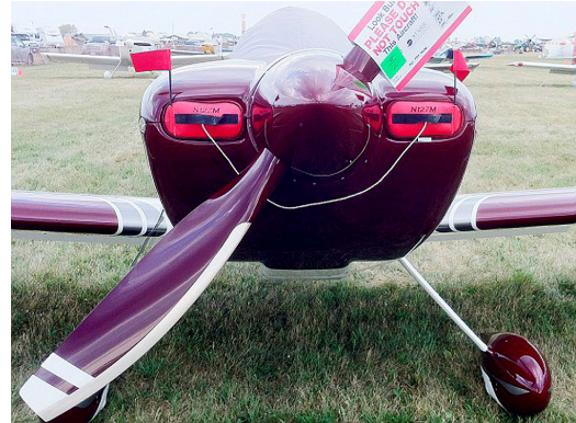
Van's RV-8 Engine Inlet Plugs
