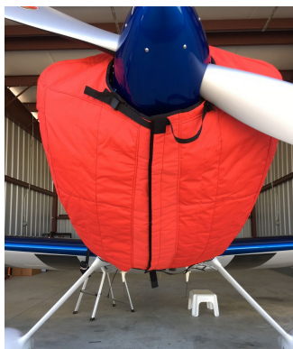
Van's RV-8 Insulated Engine Cover with Oil Filler Preheater access flap
