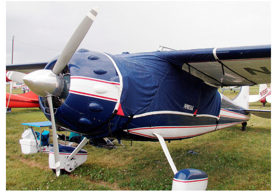
Cessna 195 Canopy Cover, extended forward and over gas caps
