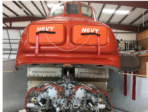
Sikorsky S58T Engine Inlet Plugs
