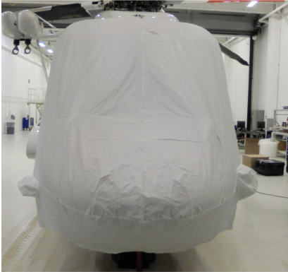
Sikorsky S-92 Windshield/Nose Cover, test fit cover
