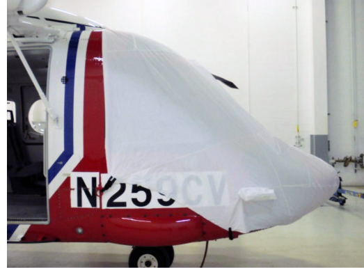
Sikorsky S-92 Windshield/Nose Cover, test fit cover
