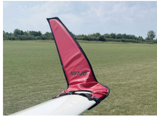
Schempp-Hirth Ventus-2B winglet/wingtip pads
