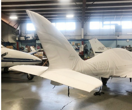
Shark 600 Complete Cover Set, test fit
