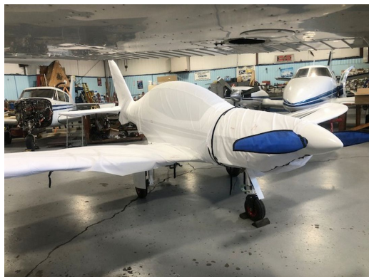
Shark 600 Complete Cover Set, test fit
