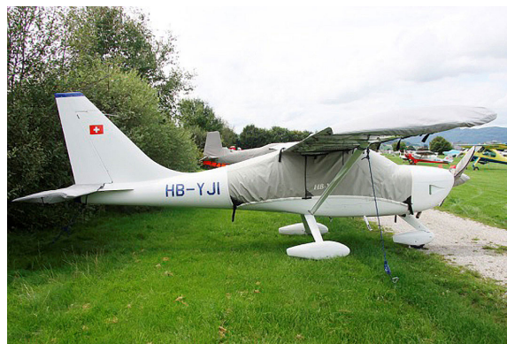
Glastar Canopy, Wings, Horizontal Stab. & Prop Covers
