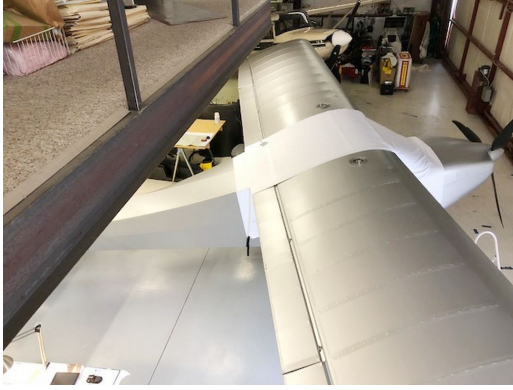
Rans S-20 Canopy Cover, test fit cover
