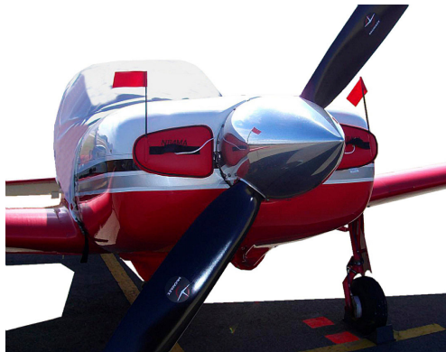
Micco SP20 Canopy Cover & Engine Inlet Plugs
