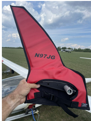
Schempp-Hirth Ventus-2B winglet/wingtip pads
