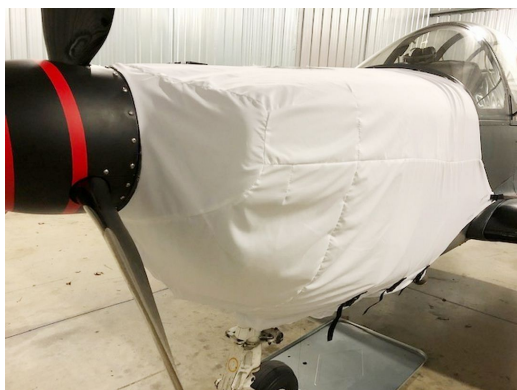
Socata Epsilon TB-30 Insulated Engine Cover, test fit cover
