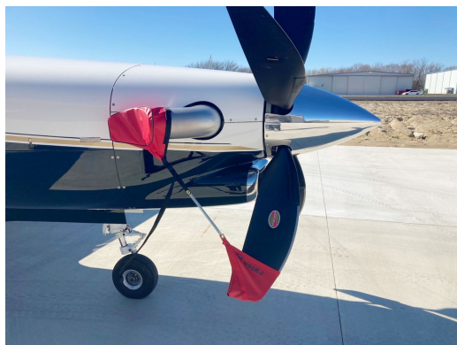
TBM 900 Prop Tie/Exhaust Covers
