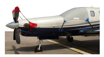
TBM700 Cockpit Cover, Engine Plugs, Prop Tie/Exhaust Covers
