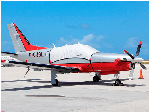
TBM Canopy Cover, Prop Tie/Exhaust Covers
