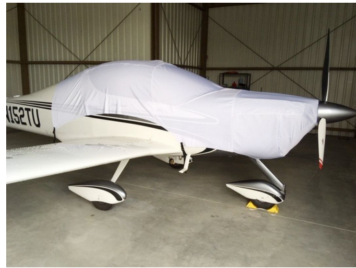
Tecnam Astore Canopy/Engine Cover, test fit cover
