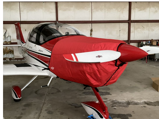
Tecnam Astore Insulated Engine Cover
