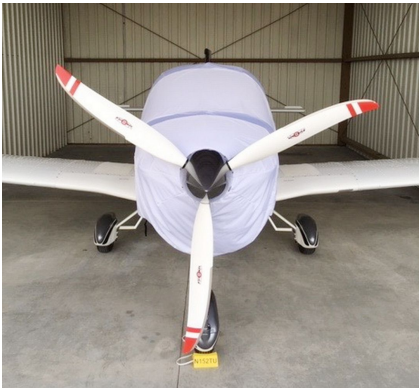
Tecnam Astore Canopy/Engine Cover, test fit cover
