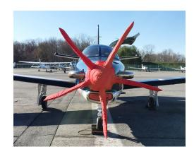
Socata TBM Insulated 5-Blade Prop/Spinner Cover
