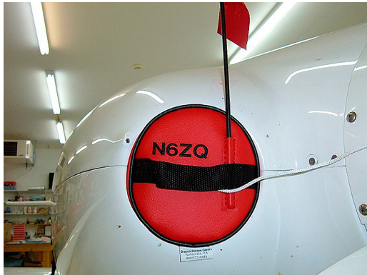
Lancair 320 Engine Inlet Plugs
