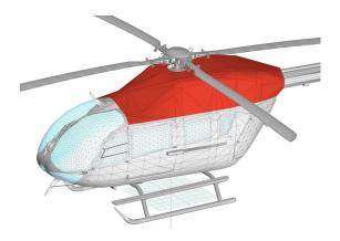
Intake/Exhaust Engine Area Cover, 3D Rendering
