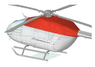
Intake/Exhaust Engine Area Cover, 3D Rendering
