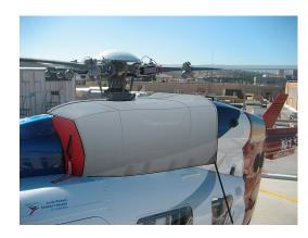
Bubble Cover w/ nose mounted radome, Upper Deck Plugs/Cover Upper Deck Plugs/Cover, extended to cover aft intake vents
