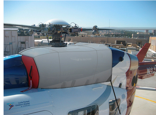
Bubble Cover w/ nose mounted radome, Upper Deck Plugs/Cover Upper Deck Plugs/Cover, extended to cover aft intake vents
