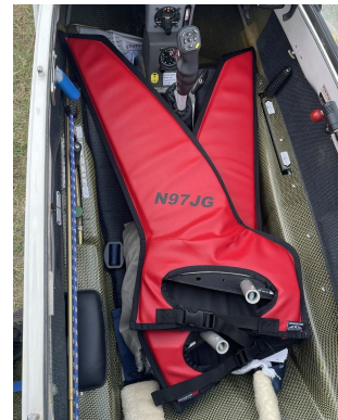
Schempp-Hirth Ventus-2B winglet/wingtip pads
