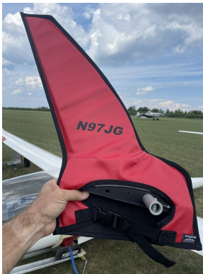
Schempp-Hirth Ventus-2B winglet/wingtip pads
