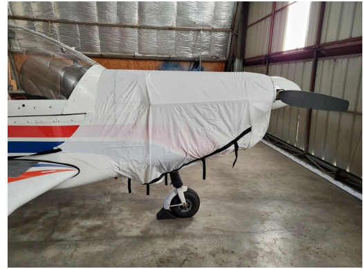
Zlin 142C Engine Cover, test fit cover
