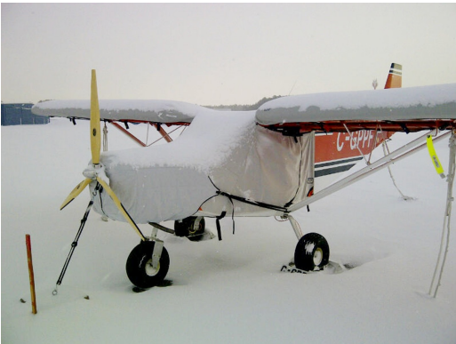
Zenith 701 Canopy, Wing, Tail & Insulated Engine Covers
